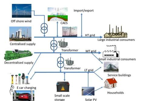
Figure 2: Schematic illustration of the electricity system represented in OPERA, including electricity infrastructure and storage
