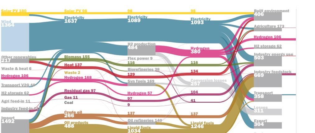
Figure 56: OPERA: Sankey diagram of the energy system in the Netherlands in NM2050
