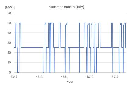
Figure 17: COMPETES: State of charge of electricity storage by Li-ion batteries in NM2050
