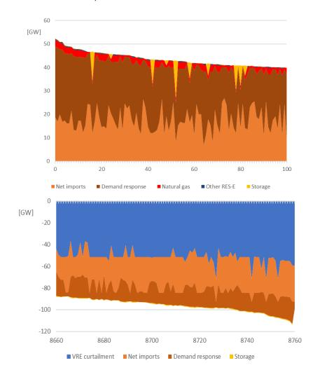
Figure 12: COMPETES: Flexibility options during the first 100 ('peak') and last 100 ('off-peak') hours of the residual load duration curve in NM2050
