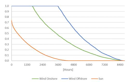
Figure 5: Duration curve of hourly capacity factors for solar PV and wind in 2050
