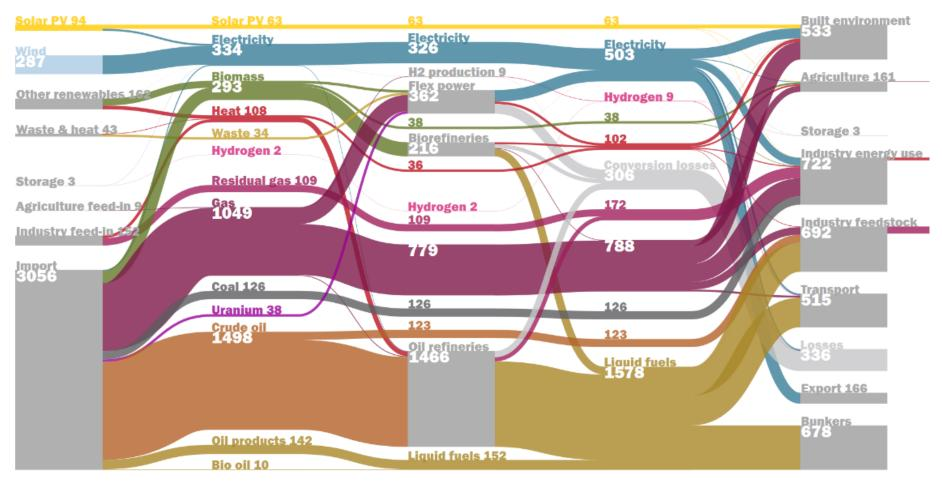
Figure 55: OPERA: Sankey diagram of the energy system in the Netherlands in CA2030
