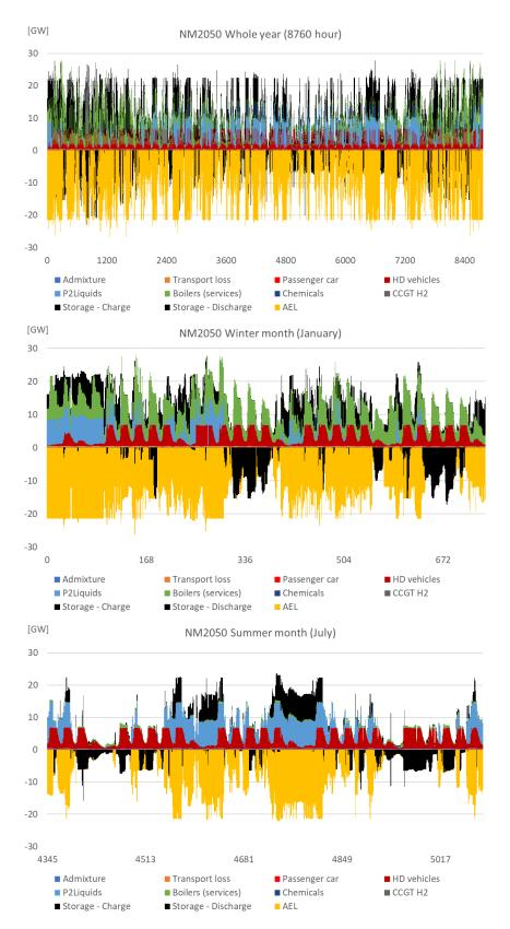
Figure 36: OPERA: Cumulative hourly profiles (stacked columns) of different categories of  ${\rm H_2}$  demand, supply and storage in NM2050
