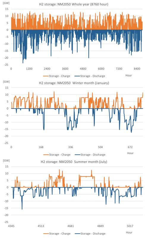
Figure 54: OPERA: Hourly profiles of H<sub>2</sub> storage in NM2050
