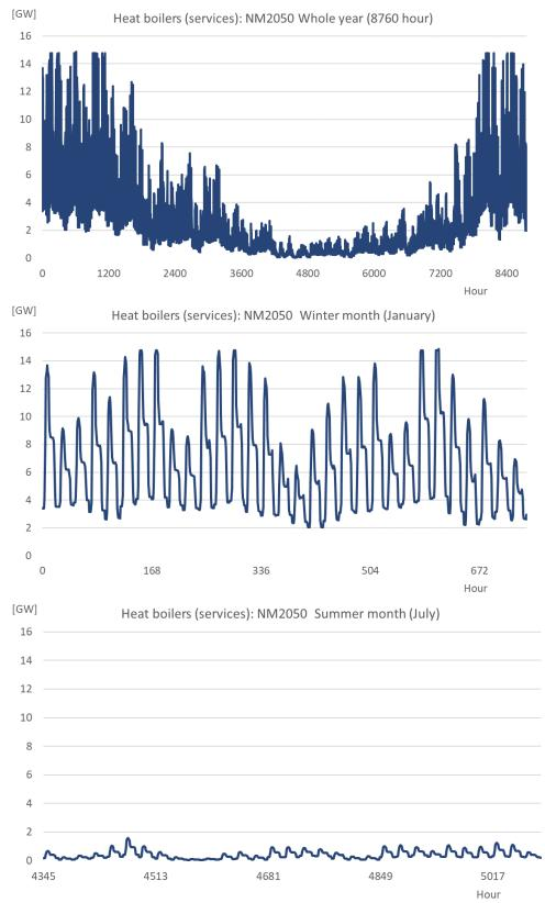
Figure 50: OPERA: Hourly profiles of H<sub>2</sub> demand by heat boilers (services sector) in NM2050
