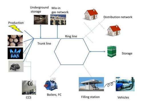
Figure 3: Schematic illustration of the hydrogen system represented in OPERA, including hydrogen infrastructure and storage
