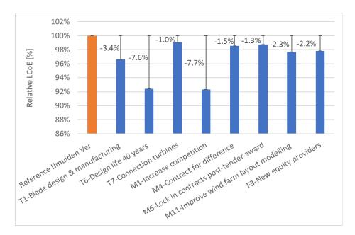
Figure 4 Relative LCoE of eight high-impact quantifiable innovations compared to reference IJmuiden Ver
