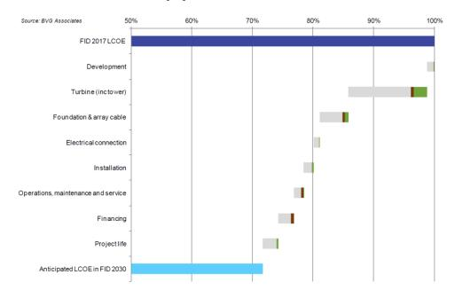
ECCE benefit from other sources Direct LCCE benefits from ports and vessels Indirect LCCE benefits from ports and vessels Figure 11 LCOE change between FID 2017 and FID 2030 at a typical reference site showing effect of port and vessel developments, from [24]
