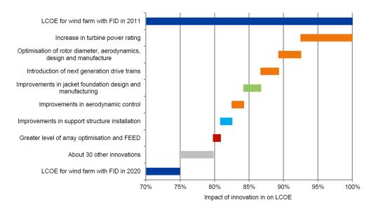
Figure 5 Anticipated impact of technology innovations for a wind farm using 6MW-Class turbines with FID in 2020, compared with a wind farm with 4MW-Class turbines with FID in 2011, from [18]
