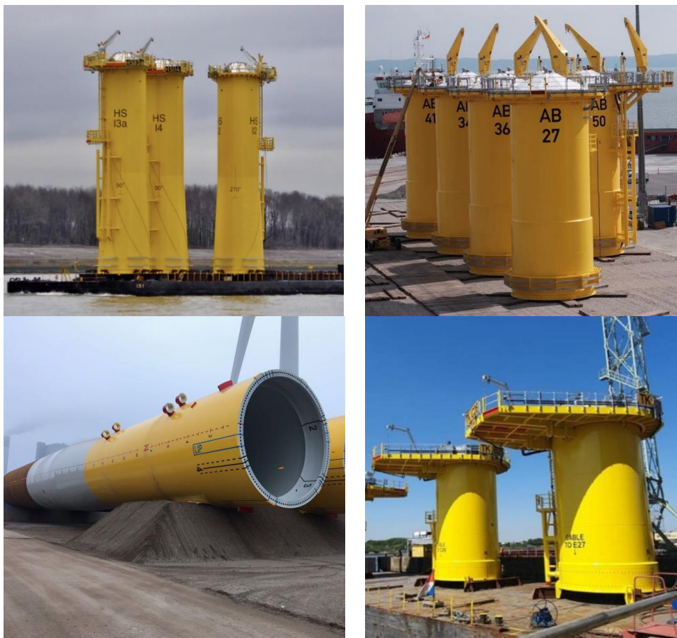
Figure 6 Examples of MP/TP variants. Clockwise from top left: grouted (Hohe See, EnBW), conventional bolted (Arkona, E.ON), compact bolted (Triton Knoll, RWE innogy), and “TP-less” monopile (Hollandse Kust Zuid 1-4, Vattenfall).
