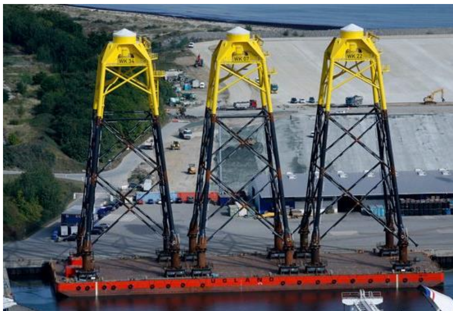
Figure 10 Four-legged jackets en-route to the Wiking wind farm (source: Iberdrola).
