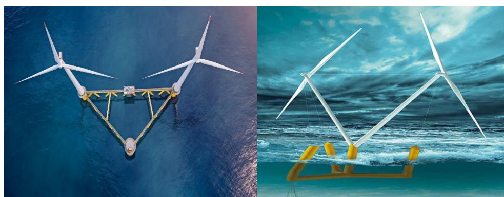
Figure 32 Floating foundations with multiple rotors: Hexicon's TwinWind and Aerodyn's Nezy2 (source: suppliers' websites).
