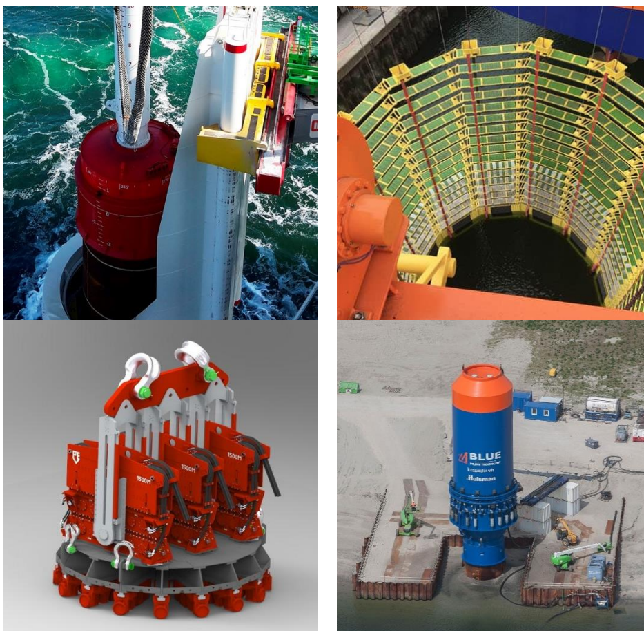
Figure 9 Examples of piling technology. Clockwise from top left: IQIP's "Integrated Monopile Installer" noise mitigation system, AdBm/Van Oord's "Noise Abatement System", IQIP's Blue Piling technology and PVE's vibro hammer (source: suppliers' websites).
