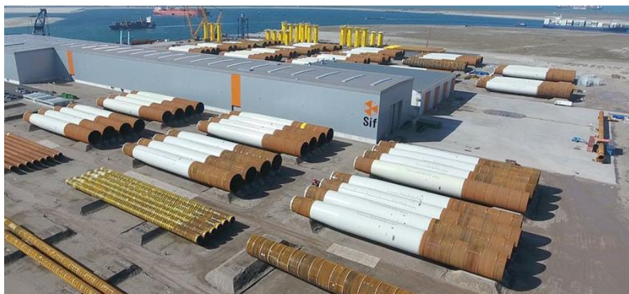
Figure 4 MP laydown post-manufacture at Sif's MP manufacturing plant at Maasvlakte 2, Rotterdam (Source: Sif).
