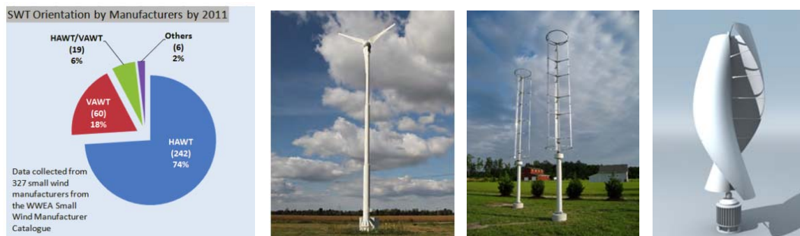
Figure 1. Left: Share of different wind turbine types in the world market (Small Wind World Report 2017). Middle: Horizontal axis wind turbine by Tuge Energia and vertical axis wind turbine (Darrieus type) by Windspire. Right: Vertical axis wind turbine (Savonius turbine)
