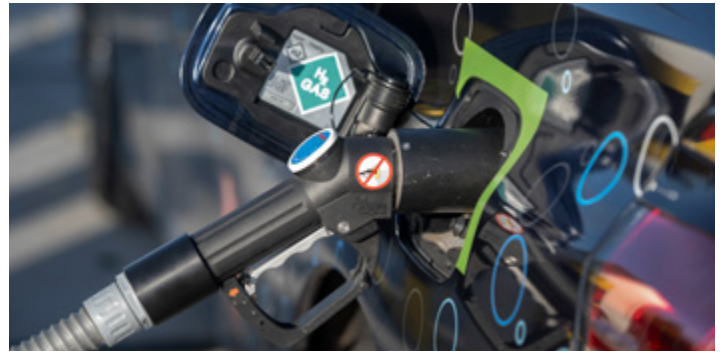
Large-scale adoption of hydrogen as a transport fuel requires new technology for filling stations. Several companies, including HyET and Resato, have developed proven solutions for some of the related challenges, such as the need for affordable and reliable high-pressure compressors.
