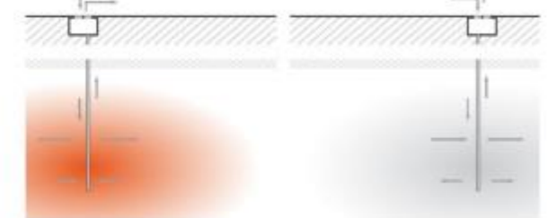
Aquifer thermal energy storage (ATES)
