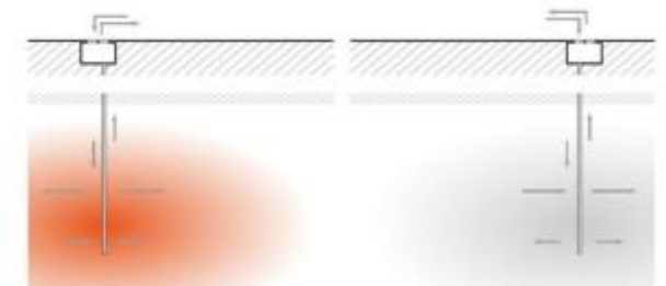
Aquifer thermal energy storage (ATES)
