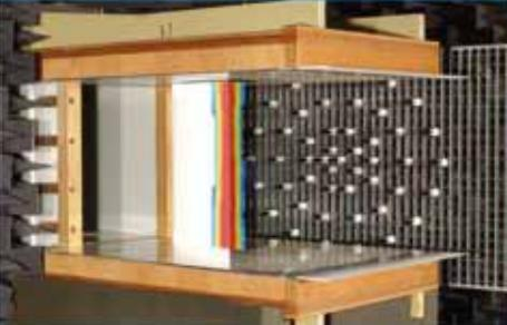
**Acoustic wind tunnel tests**
